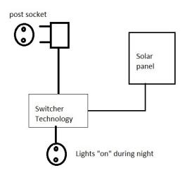
Using a Switcher technology, the device senses light condition using solar panel. The bigger the solar panel, the more sensitive and accurate turning on and off of the lights.
